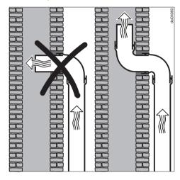
If the exhaust air is to be ducted into a vent flue, the ducting must be directed in the flow direction of the flue.
